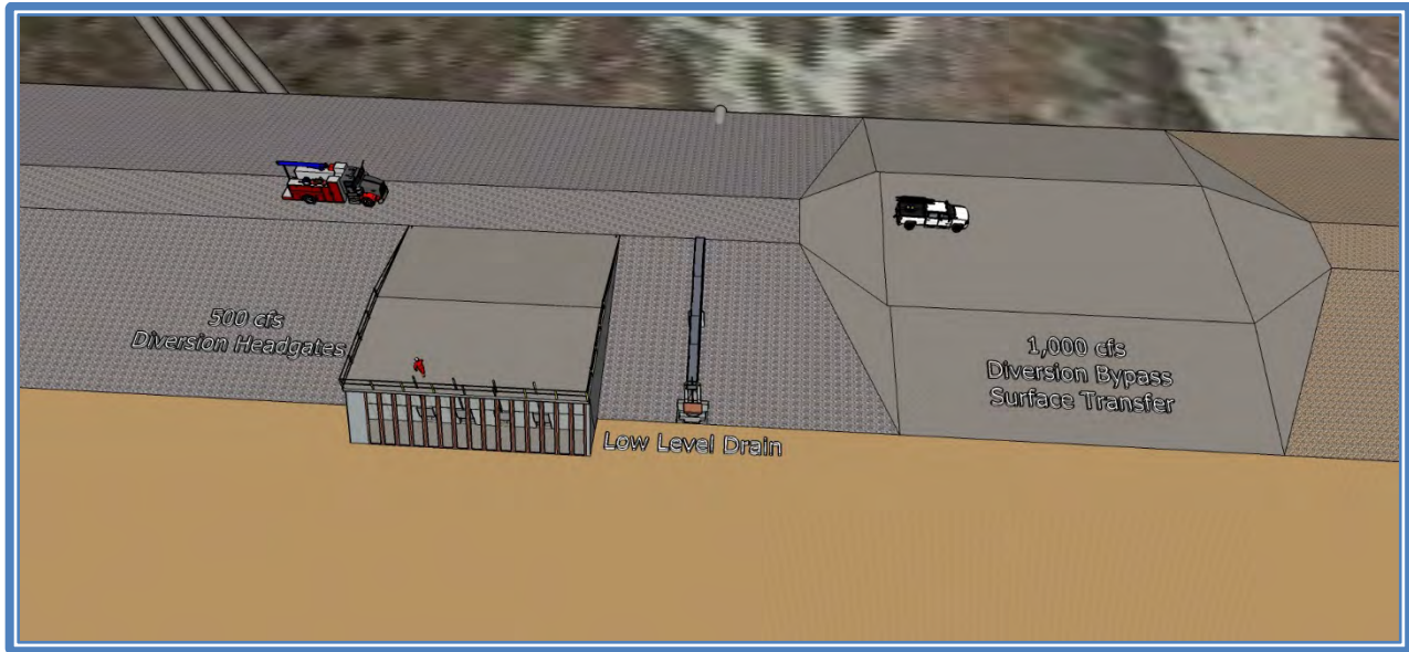
Figure 109: Cajon Creek/Vulcan 1 Basin Conceptual Design (Diversion View)
