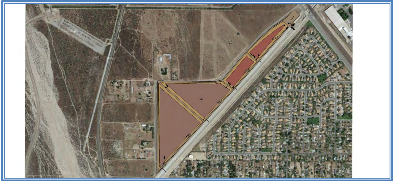
Figure 118: Vulcan 2 Basin Conceptual Design (Plan View)
