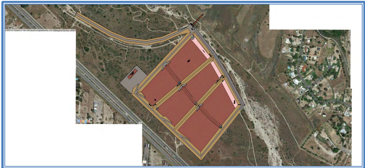
Figure 78: Cable Creek Basin Conceptual Design (Plan View)
