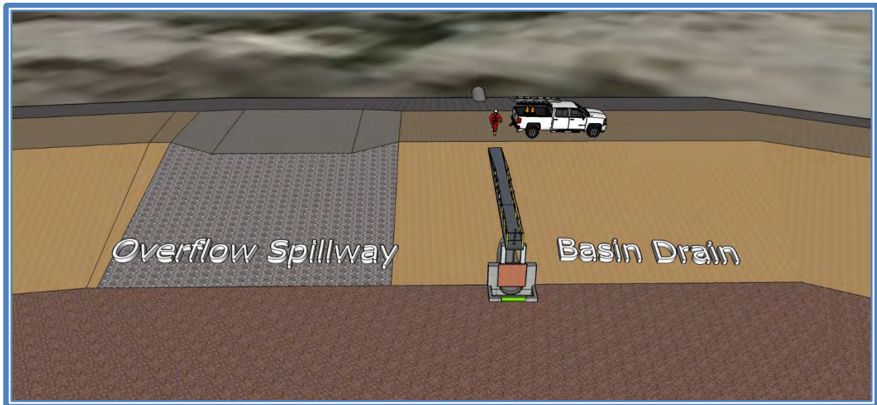
Figure 21: Plunge Creek Basin 1 Conceptual Design (Basin Outlet)
