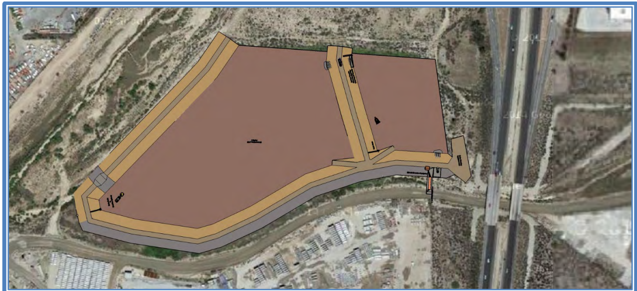
Figure 28: Plunge Creek Basin 2 Conceptual Design (Plan View)
