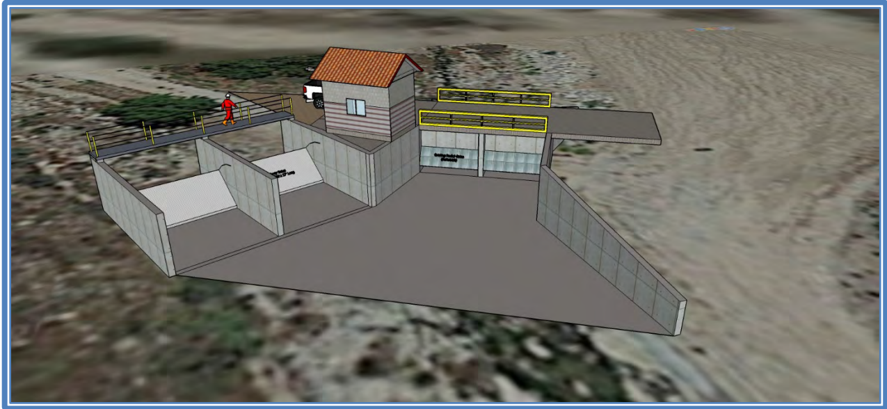
Figure 49: Waterman Basins Conceptual Design (Diversion Isometric View)
