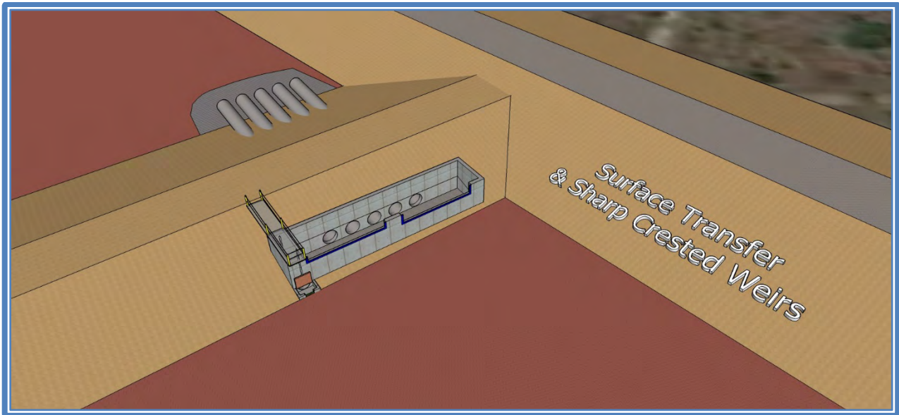
Figure 80: Cable Creek Basin Conceptual Design (Transfer Structure View)
