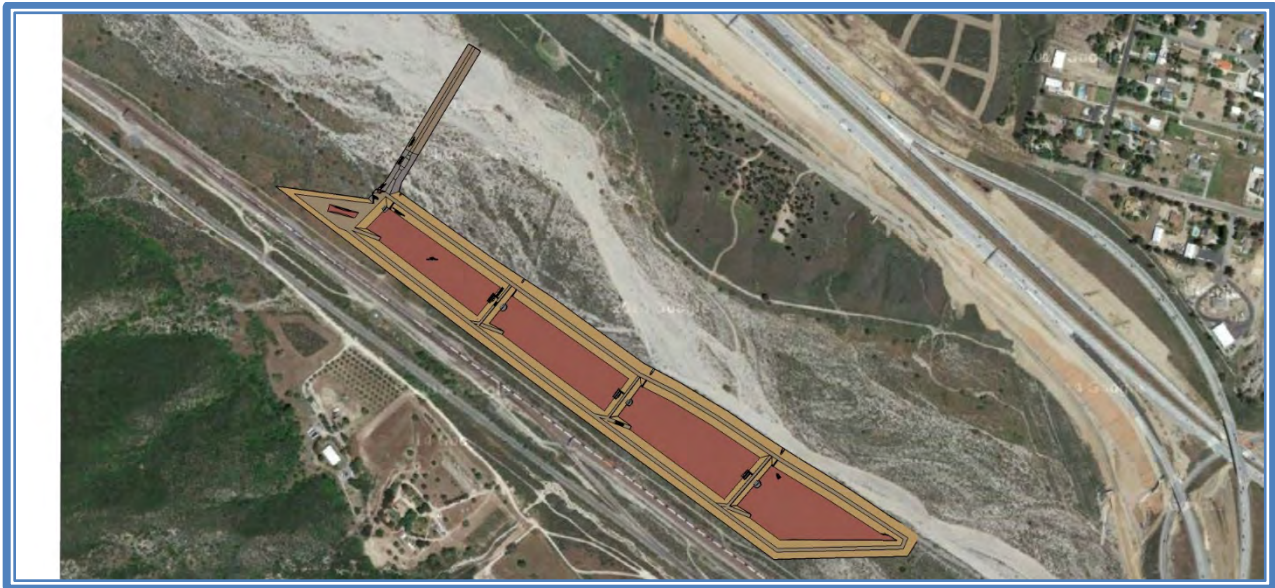
Figure 98: Cajon Creek Basin Conceptual Design (Plan View)
