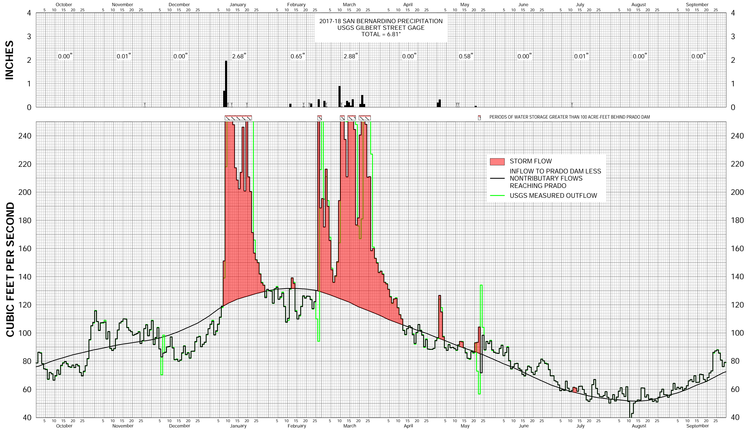
DISCHARGE OF THE SANTA ANA RIVER AT PRADO DAM & SAN BERNARDINO PRECIPITATION WATER YEAR 2017-18
