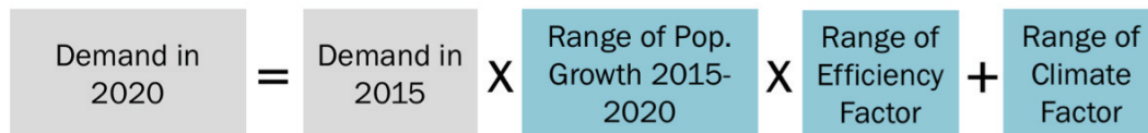
Figure 5. Updated unit water demand model with additional factors to reflect key drivers of demand
