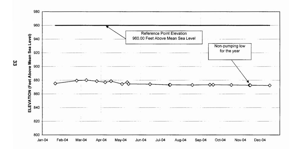
FIGURE 2 **GROUNDWATER SURFACE ELEVATIONS FLUME NO. 2 WELL** 2004
