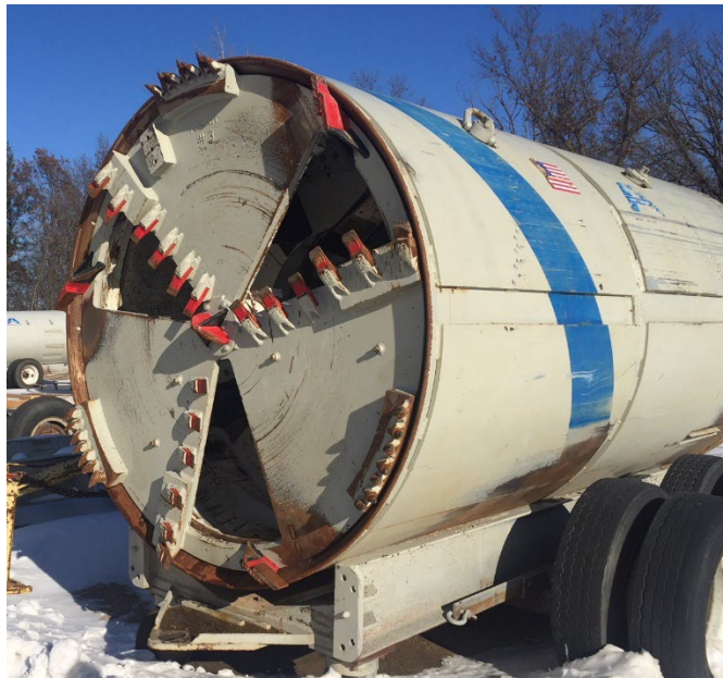
Figure 9 Open-Face Pipe Jacking Shield with Iris Doors
