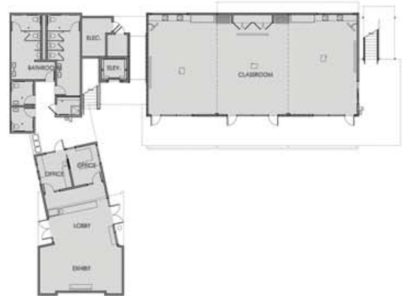
CLASSROOM BUILDING FIRST FLOOR PLAN
