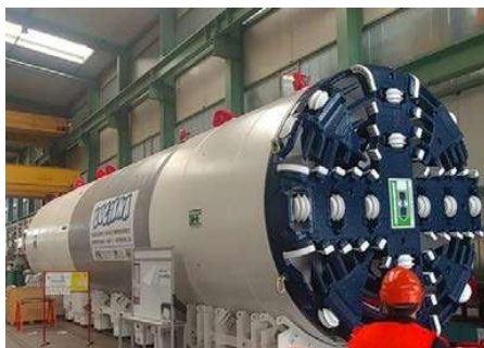
EPB TBM of Tunnel Segment 10.
