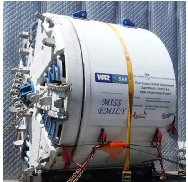
Part of EPB TBM used in tunneling in RSC Units 5 & 6.
